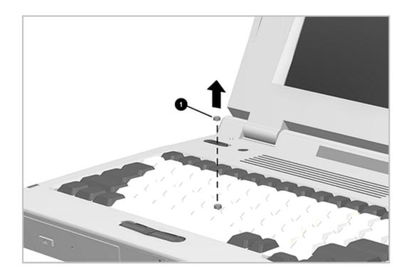
Figure 5-19. Removing and Installing the EasyPoint II Pointing Device
